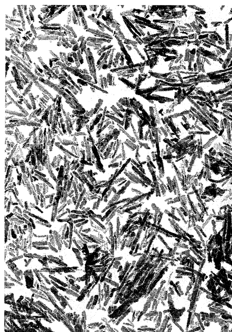
Fig. 1. Electron micrograph of the original iron powder ( \times 15000 ).
